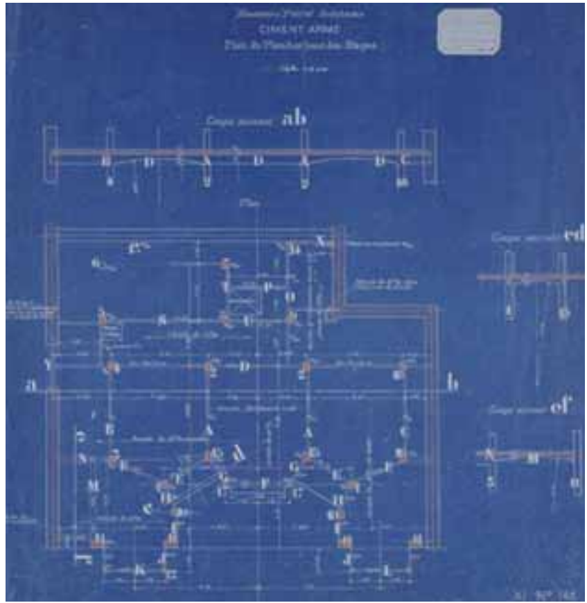
Blueprint. Auguste Perret, Concrete plan for typical floor, building at 25 bis, rue Franklin, Paris 16 e .
