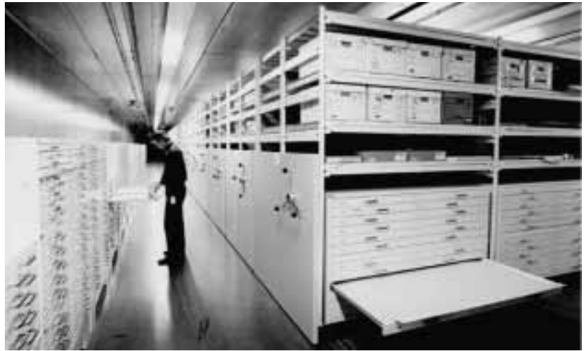
Architectural drawings and map drawer filing cabinets, stacked. Note the cabinet bases; the offset handles; the drawers containing one or two side-by-side piles of folders; the movable flap at the front of each drawer.
